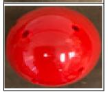
Use a soldering iron to burn the small sound holes in the top (allows sound to emanate).
